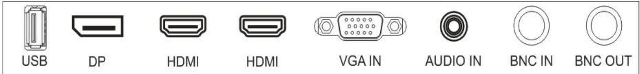
VGA INPUT: D-SUB 15 pins Connector
